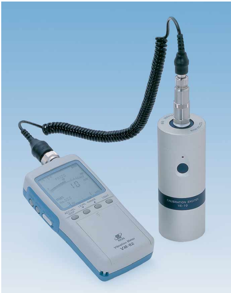
Calibration of Vibration Meter VM-82 by VE-10
